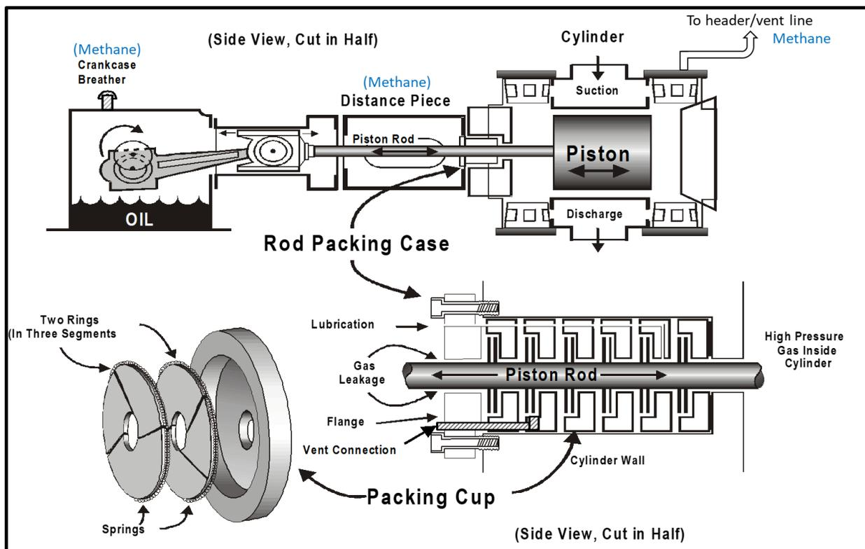
The volume of emissions from the compressors depends on cylinder pressure, fitting and alignment of the packing parts during assembly, and amount of wear on the rings and rod shaft. Packings of reciprocating compressors allow some gas escape (leak), including newly installed compressors. This amount increases as the system ages. Replacement of the packings in a timely manner is part of a good maintenance.
